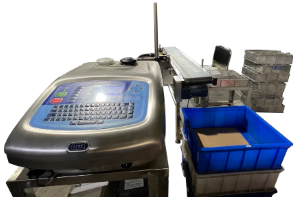
Figure 4-3 "LINK5900" type inkjet machine
